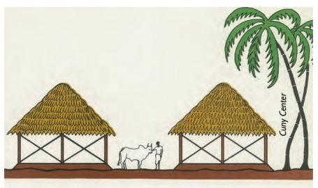
Shelter design elevation showing cross-bracing
