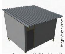
Computer model of the shelter with a corrugated iron roof and plastic sheeting
