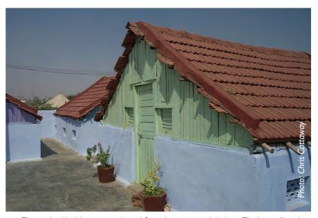
These school buildings were adapted from the transitional shelters. The low walls reduce the risk of masonry falling on occupants during future earthquakes.
