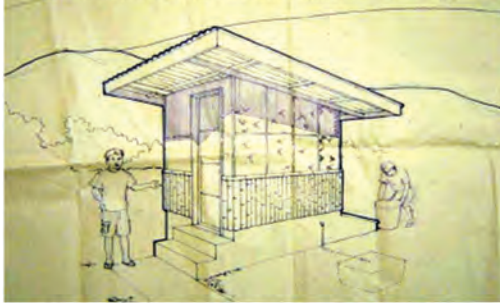
Double-vault dehydration toilets, Bohol, Philippines
