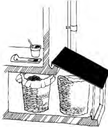
Figure 13: A single-vault, solar-heated eco-toilet with moveable containers, in this case two large baskets. When the first basket is full it is placed directly under the solar heater and remains there until the second basket is full
