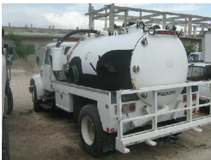
A sludge tanker
